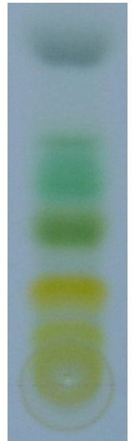
Thin layer chromatography is used to separate components of chlorophyll
